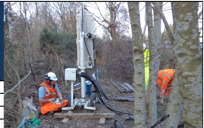
Above & Below: Modular Window Sampling Rig
