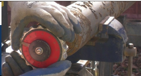
Left: Shear vane in windowless sample
